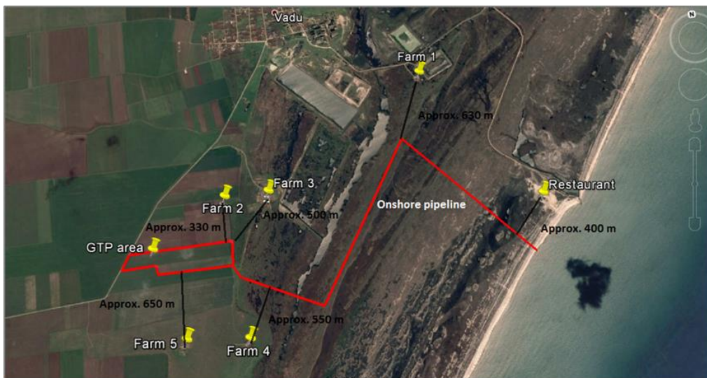
Figure 2 Settlements and structures located near MGD
